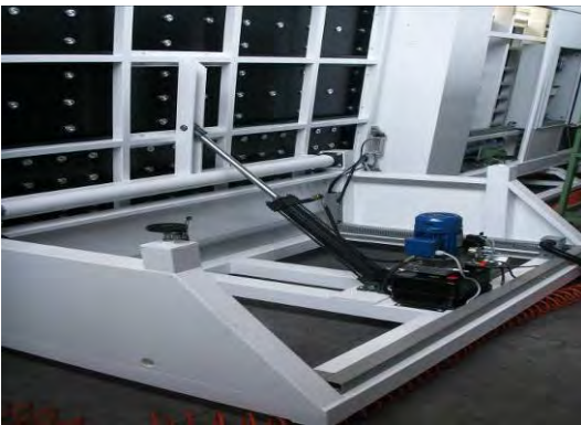
Optional hydraulic tilting table system
