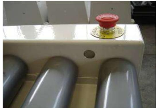
01 Motorized exit with a length of 2 mt. and height of 0,90 mt., with clutched anticut vulcollan rollers, mounted on bearings and bushing in special plastic material. This module has a motor complete of reducer. The four blowers are fed by one high pressure fan , stop glass system through sensor. Protections against access to the dangerous parts of the machine according to the EU norms.
